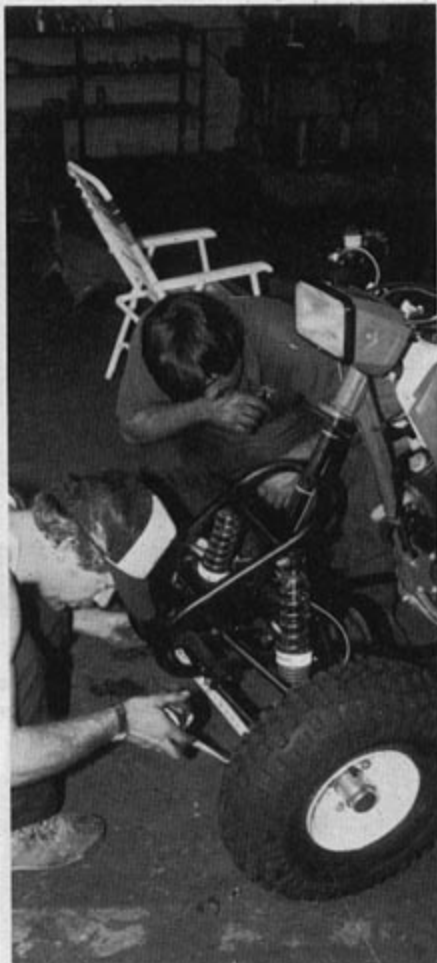
Part of the installation includes setting the toe in. We set ours at about 1/4-inch using a tape measure and adjusting the tie rods ends.
