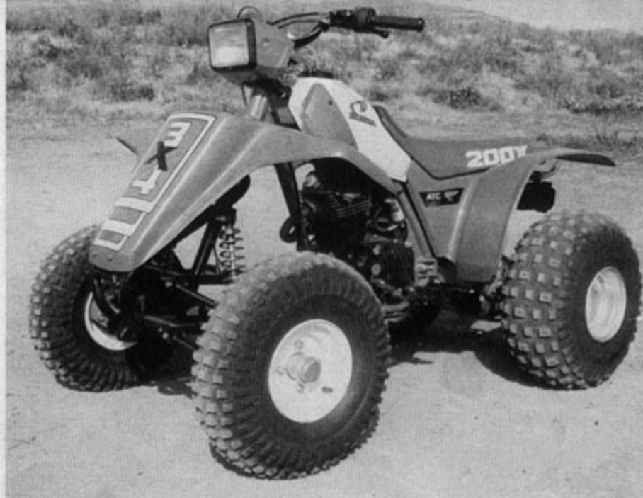
Although the 3X4 kit installs easily and makes the 200X a true 4-wheeler, the front fender looks out of place on the Honda.
