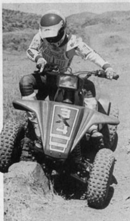
ABOVE RIGHT, equal length A-arms use car-type tie rod ends and new spindles. ABOVE, with small front tires, ground clearance is limited.
