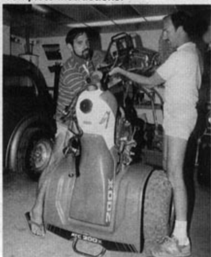
The complete 3X4 assembly bolts on with only a few tools. A special wrench is supplied for the steering head along with a good set of complete instructions.
